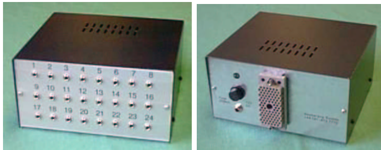
Figure 3: Custom microphone power box (front and rear)
